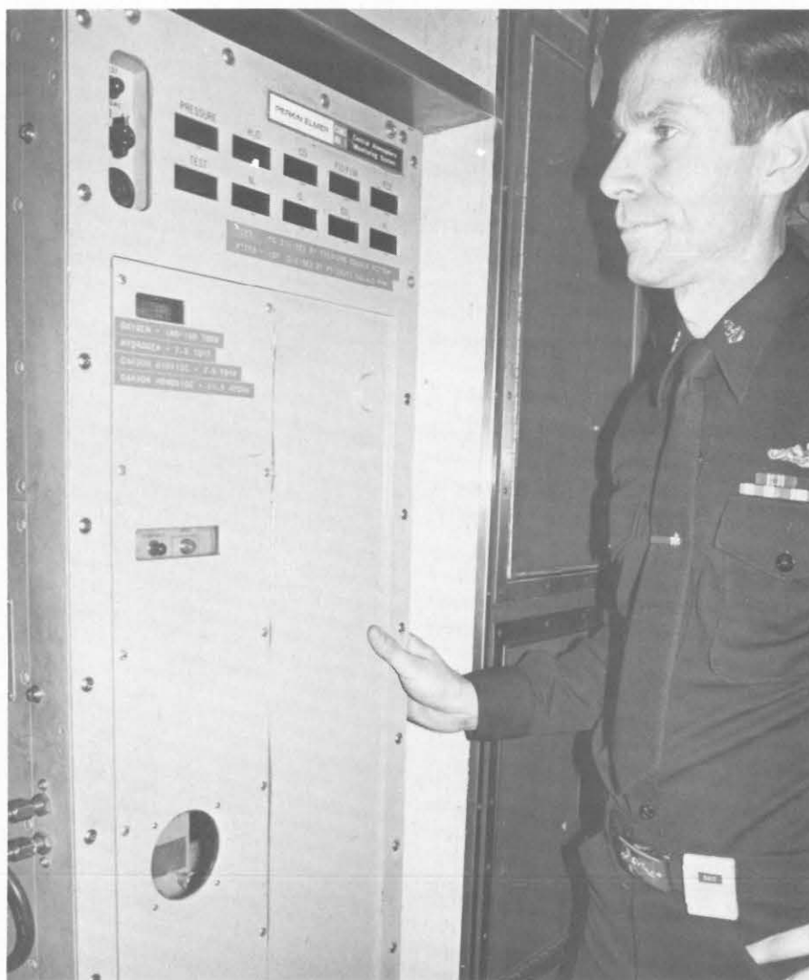
A submarine corpsman's responsibilities include the monitoring of the vessel's atmosphere. The CAMS (Central Atmosphere Monitoring System) tests for levels of oxygen, carbon dioxide, carbon monoxide, hydrogen, and nitrogen.
